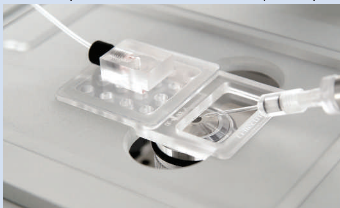
Cellectricon's Dynaflow patch-clamp system combines microfluidics and patch-clamping technology.
